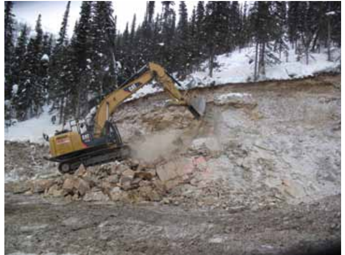
A backhoe extracts gold-rich material from the Sleeping Giant Zone at the 3 Aces Project in the Yukon for the bulk sample. Photo courtesy Golden Predator Mining Corp.
