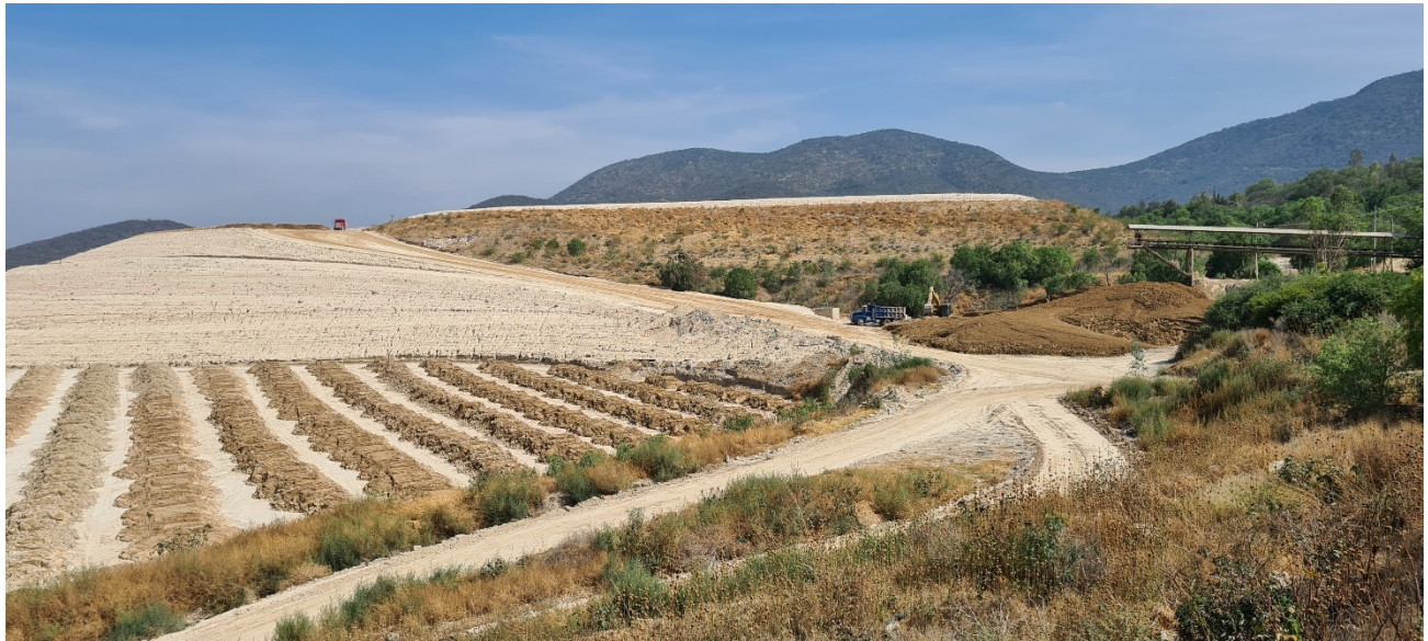
Figure 14-2: Dried tailings being collected and hauled to the tailings dam
